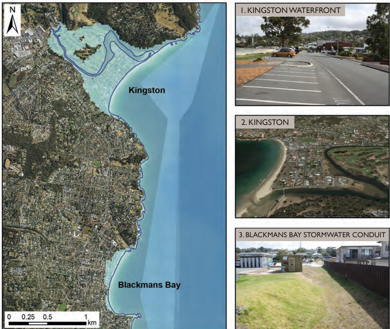
FIGURE 10: Maximum modelled inundation extent at Kingston and Blackmans Bay. A stormwater drainage conduit is present at Blackmans Bay and could result in inundation distances that are greater than predicted.
